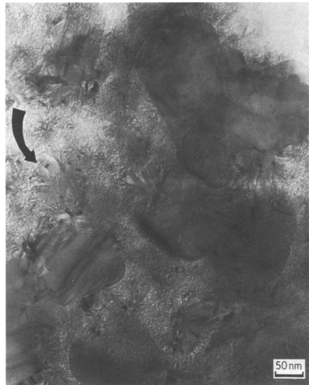
Figure 7 Graphite spherulites (arrowed) surrounding SiC crystals.
